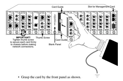
• Insert the card into a slot in the chassis making sure that the top and bottom edges of the board are aligned with the top and bottom card guides in the chassis. Do not force the card into the chassis unnecessarily. It should slide in easily and evenly.
